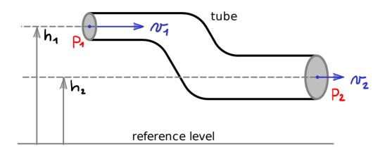
In a tube with flowing liquid the pressure, velocity and level change at each point but the following their combination remains constant:
