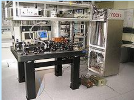
FOCS 1, a continuous cold caesium fountain atomic clock in Switzerland, started operating in 2004 at an uncertainty of one second in 30 million years.
