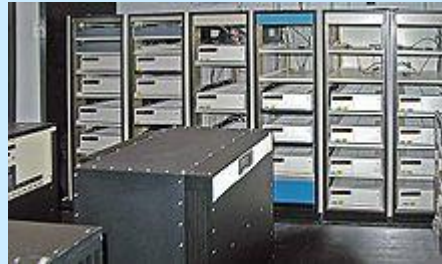
The master atomic clock ensemble at the U.S. Naval Observatory in Washington D.C. , which provides the time standard for the U.S. Department of Defense.
