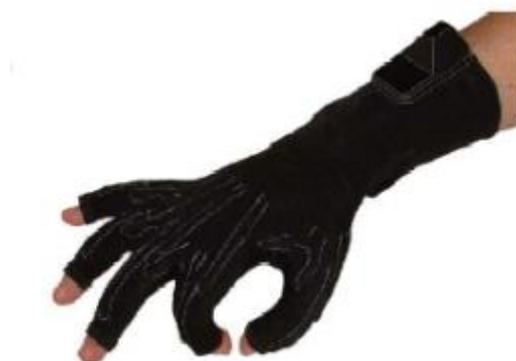
A first approach to integrate electronics into textile structures was certainly achieved by gloves wired to the computer that allows it to take input from user's hand gestures. Sensors in the glove detect (Figure 11) the wearer's hand movements. Four wires were used for each finger or tube to build up a circuit. The voltages coming out are varying depending on the finger position [65].
