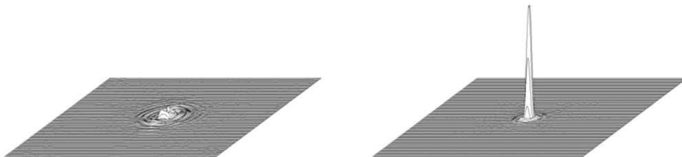
Fig. 3. PSFs before (left) and after (right) correction with the 37-actuator FDM. Wavelength used is 659.5 nm and Strehl ratio of corrected PSF is 0.84.
