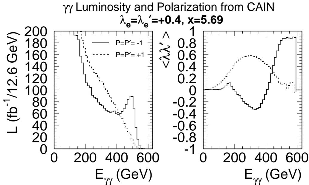
Figure 3: Yearly luminosity in units  $\text{fb}^{-1}/12.6 \text{ GeV}$  and associated  $\langle \lambda \lambda' \rangle$  are plotted for  $\sqrt{s} = 630 \text{ GeV}$  ( $x = 5.69$  for  $1.054 \mu\text{m}$  laser wavelength), assuming 80% electron beam polarizations, for polarization orientation cases (I) and (II).
