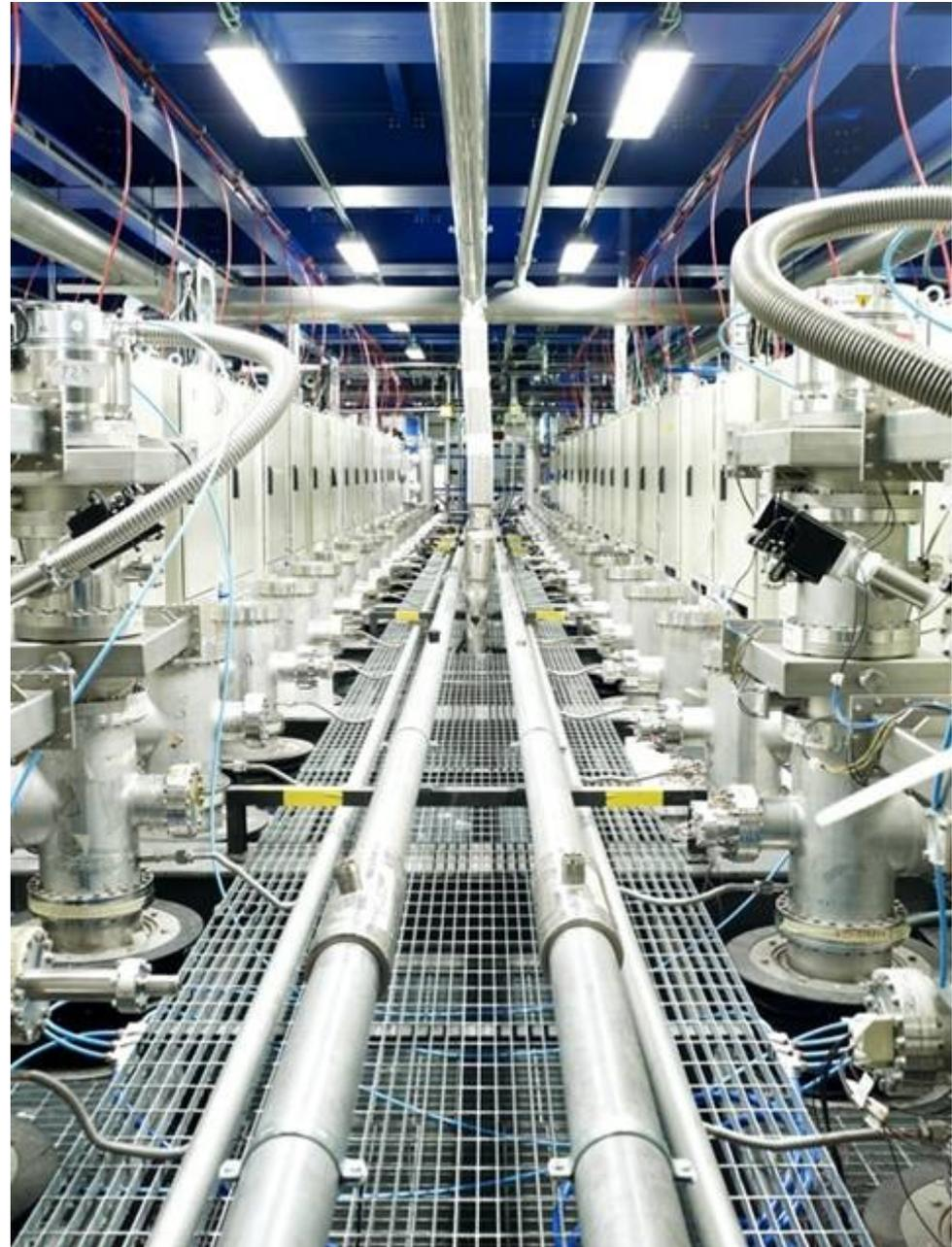
The experimental technique of the ICARUS T600 detector is based on the use of **Time Projection Chambers (TPC)** in liquid argon. The detector consists of two identical semi-modules, each hosting 300 tons of liquid argon 'observed' by two TPCs and 20 photomultipliers. This kind of detector is able to produce high granularity 3D reconstruction of recorded events as well as high precision measurements over large sensitive volumes.
