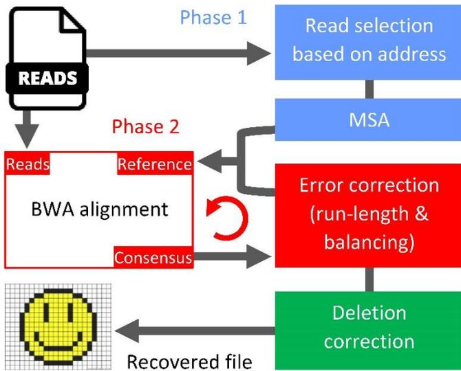
**Figure 2 | Post processing via sequence alignment and homopolymer correction.** In the first phase, an estimate of the DNA codewords is obtained by running MSA algorithms on high-quality reads that contain an exact match with the address sequence. The second phase improves the estimate by employing an iterative method that includes BWA alignment and an error-correcting scheme.
