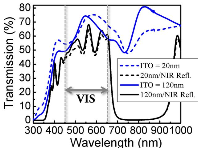
FIG. 3. (Color online) Transmission spectra of the transparent OPV devices for various ITO cathode thicknesses with, and without, the NIR reflector. The approximate visible photopic range is highlighted with vertical dashed-lines. The transmission curves for the assembled transparent OPV closely matches the transmission curve for the NIR mirror (see Ref. 12).
